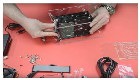
Assembling an ODROID XU4 CloudShell 2 NAS Unit
